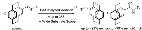
Scheme 1 Synthesis of [2.2]paracyclophane derivatives with planar and central chirality via kinetic resolution.
