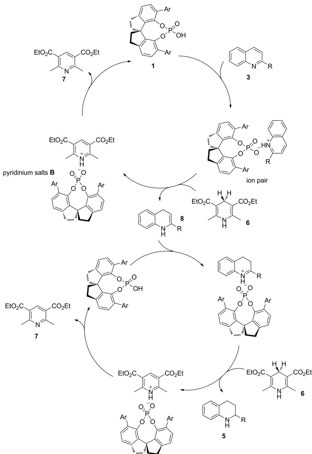
Scheme 3. Proposed catalytic cycle for the SPINOL-derived chiral phosphoric acid catalyzed hydrogenation of 2-arylquinolines **3**.
