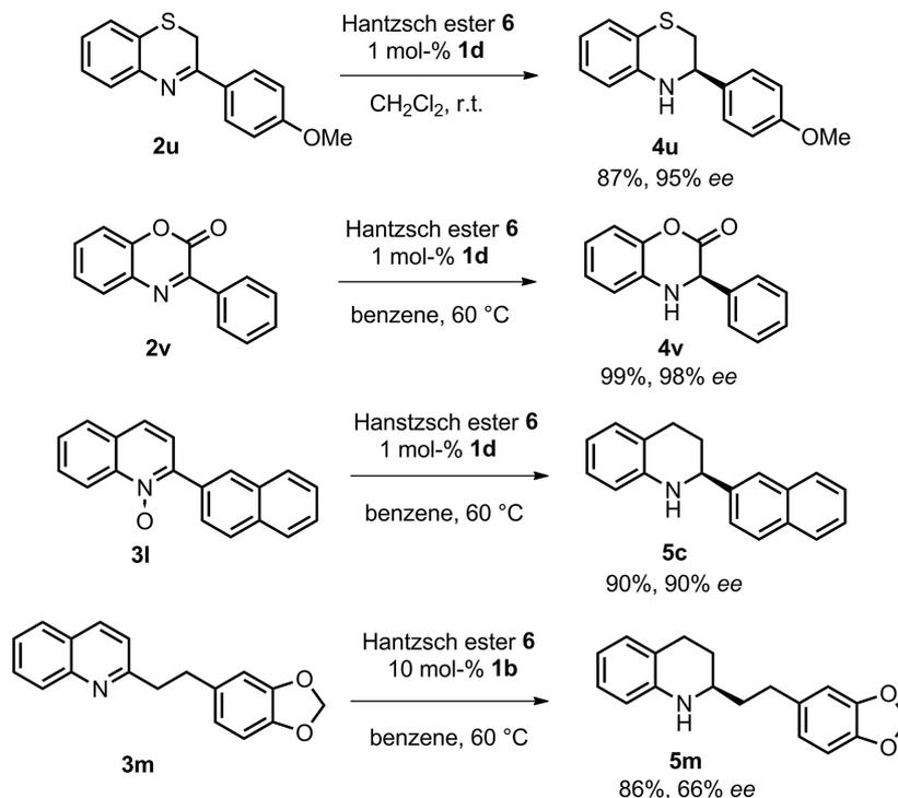
Scheme 1. Substrate scope of other transfer hydrogenation reactions.
