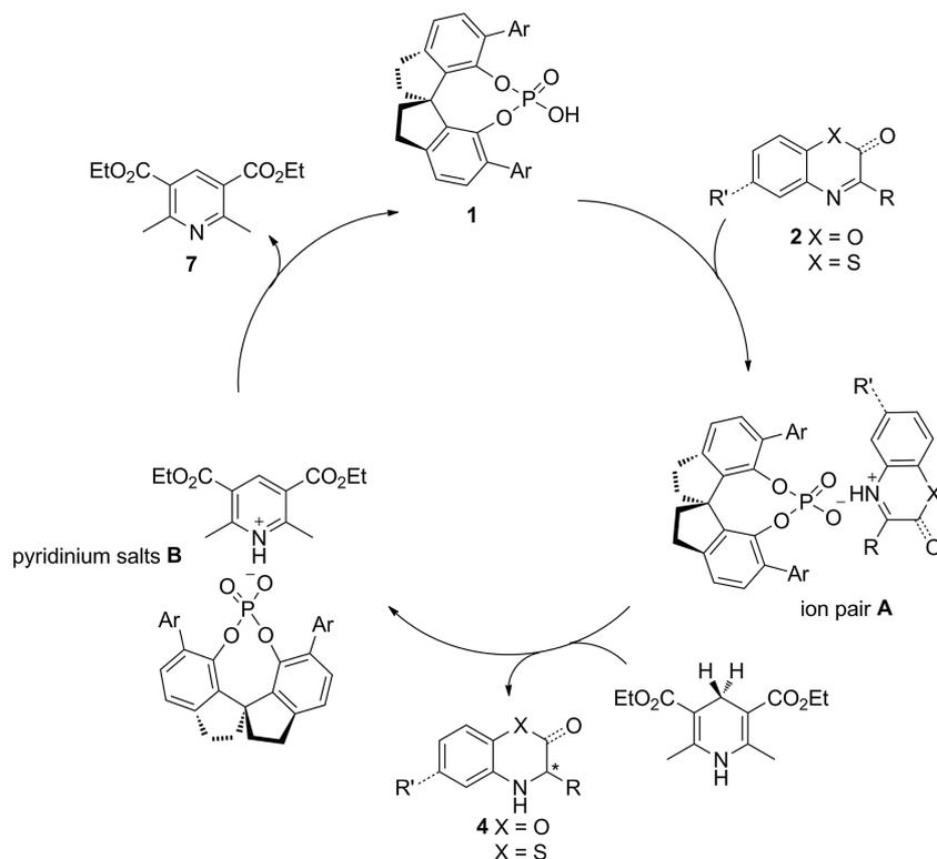
Scheme 2. Proposed catalytic cycle for the SPINOL-derived chiral phosphoric acid catalyzed hydrogenation of 3-aryl-1,4-benzoxazines **2**.
